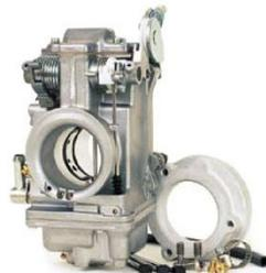
Picture 3: Mikuni HSR42 42mm Carburetor (shown with AC adapter)
